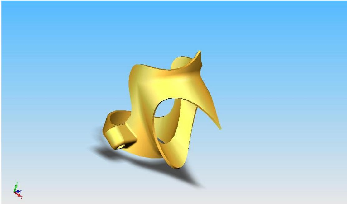
**The 3D drawing of the "Tiny Slant 6" down tube lug with integral cast gear cable bosses. Sexy curves eh! I have to frankly admit, I am quite proud of the results.**
